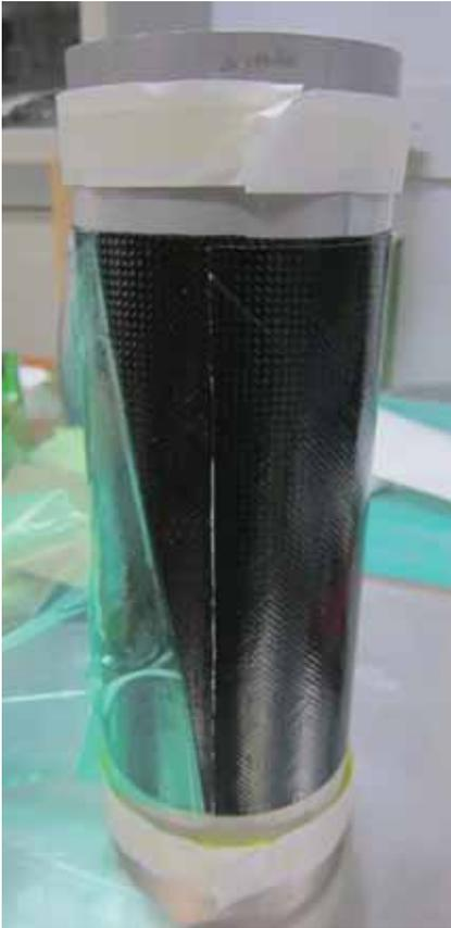
Fig. 1: CFRP plies wrapped around Al cylinder.
