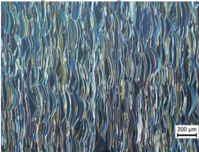
Fig. 9a. Si-face of Pure-Si grown for 5h
