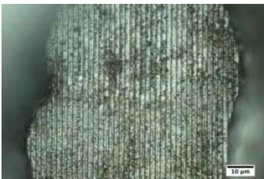
**Fig. 19) Optical plan view after n-contact deposition**
