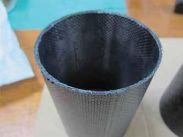
Fig. 6: Crushed end of 0/90 tube.
