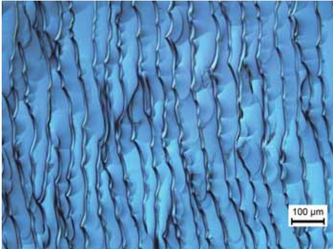
Fig. 9a. C-face of Pure-Si grown for 5h
