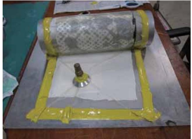
Fig. 3: Vacuum bagged tube after curing in autoclave. Note the resin that has been absorbed by the breather cloth.
