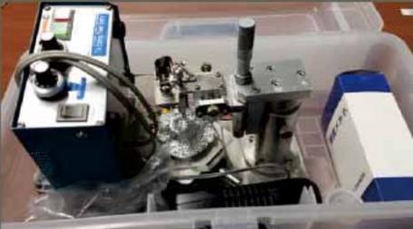
STM Tip Making Apparatus – NaOH with 0.15mm Tungsten Wire
