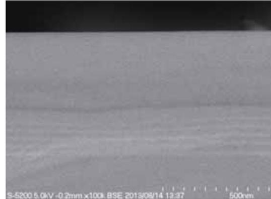
**Fig. 7) BSE SEM cross-section of LED structure**
