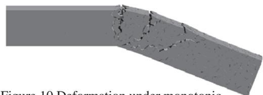
Figure 10 Deformation under monotonic loading at 20mm ( $4\delta_y$ )
