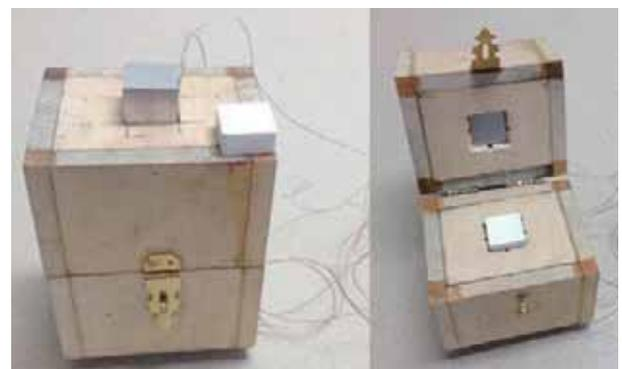
Fig. 7 Thermal Insulation Box for Thermal Conductivity Test.
